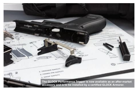
safe, even if exposed to high external forces. It is flatter in profile if viewed from the side. The firing pin safety function is retained, automatically engaging as the trigger returns forward. Finally, the drop safety, a positive mechanical connection between the trigger bar and firing pin, prevents ignition even if the pistol is dropped.
