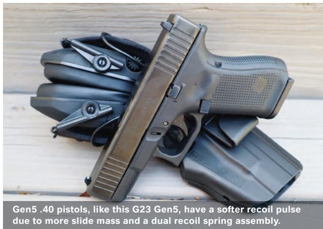
Gen5 .40 pistols, like this G23 Gen5, have a softer recoil pulse due to more slide mass and a dual recoil spring assembly.
